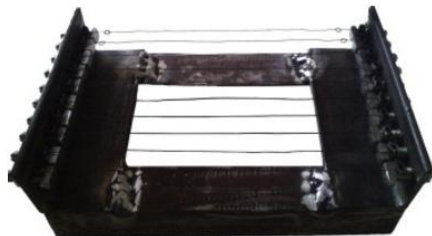
Fig 1 SMA wires straightened in fixture.
