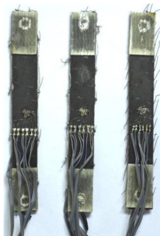
Fig 8 Oriented fibers and SMA wires in the specimens with strain rosettes.
