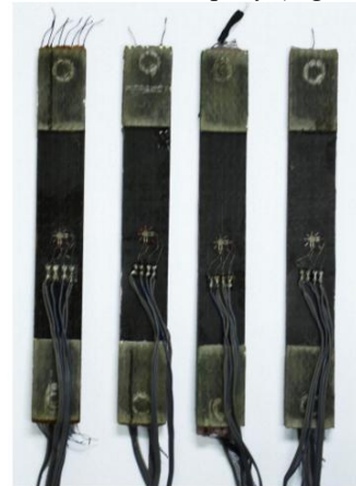
Fig 7 Unidirectional fibers in direction of tensile loading. Specimen with strain gages.
